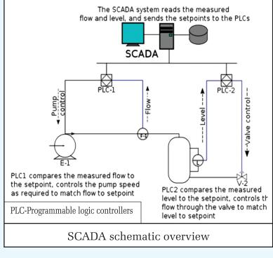
consists of servers having SCADA software and the three following elements:
