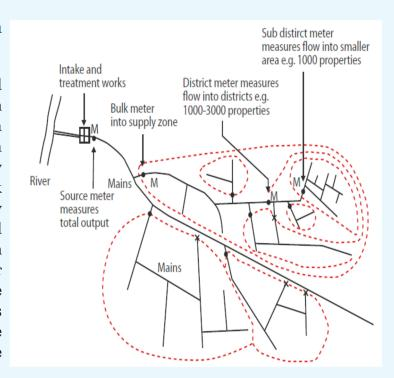
than one point as per the site requirements. Analysis of water flow and pressure, particularly in the night when most users are not drawing water enables leakage specialists to identify leakages and calculate the level of leaks in the DMA. This can be used to determine not only whether work should be undertaken to reduce leakage, also to compare levels of leakage in the different DMAs and thereby take up the required maintenance.
